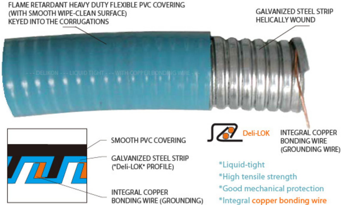
Liquid Tight Conduit With PVC Covering ( YF-604 )
