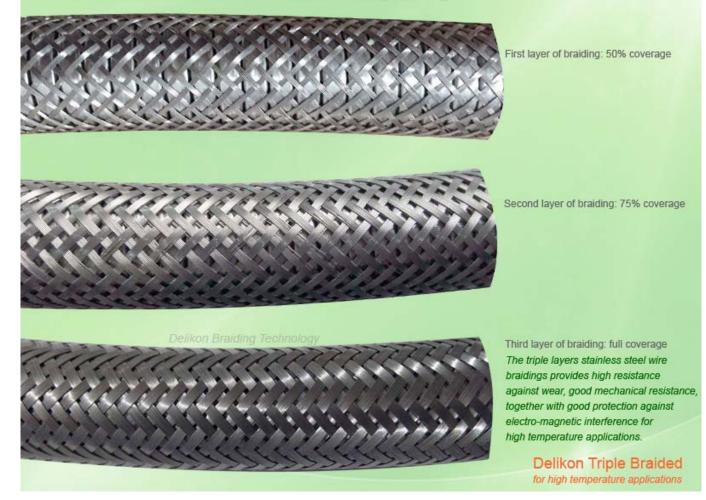
Delikon Heavy Series Triple Layers Stainless Steel Wire Over Braided Flexible Stainless Steel Conduit for combustion equipment power and data cable protection: igniters, flame detectors, Burner Management Systems (BMS) sensor and detector cables, dampers, burners and duct burners cables
