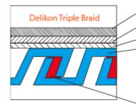
Third Layer of Stainless Steel Wire Braiding (Full) Second Layer of Stainless Steel Wire Braiding (75%) First Layer of Stainless Steel Wire Braiding (50%) Hellically Wound Stainless Steel Strip ("Deli-LOK" Profile)
